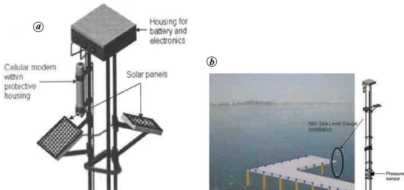
**Figure 1.** *a*, Top portion of mounting structure of the gauge, where battery, electronics, solar panel and cellular modem are fixed. *b*, Illustration of NIO sea-level gauge installed at Verem Jetty, Mandovi estuary, Goa, India.
