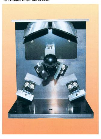
Fig. 1—Show the Diffuse Reflectance (DR) attachment used for the measurement of DRIFT spectrum
