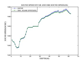
Fig.11. Sound speed (m/sec) by PMC V/S Depth (m)
