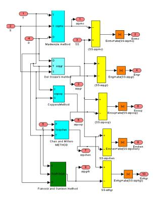
Fig.2 Sub Simulation model for sound speed showing different types of sound speed simulations
