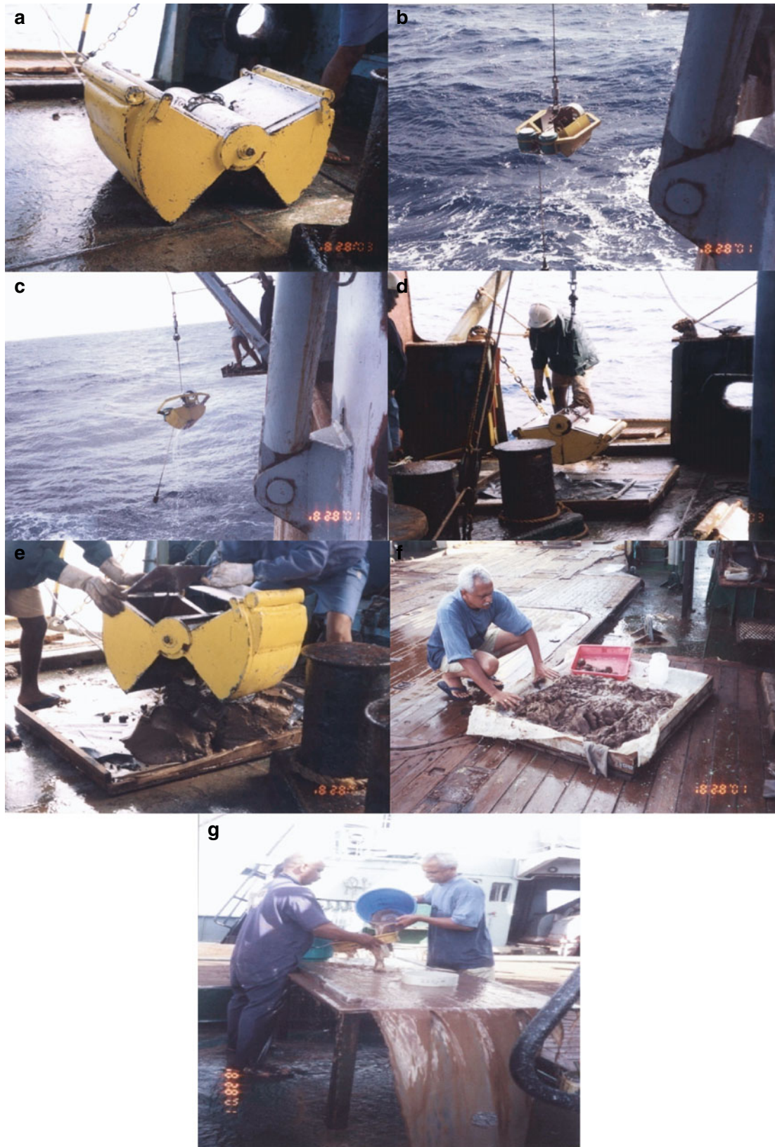
Figure 1. Sample collection by using van veen grab from the Indian Ocean basin: (a) van veen grab, (b) lowering the grab, (c) lifting up the grab from water column with the sediments, (d–e) collecting sediments from grab, (f) sediments samples collected by using grab sampler, and (g) sieving of the grab samples on board.
