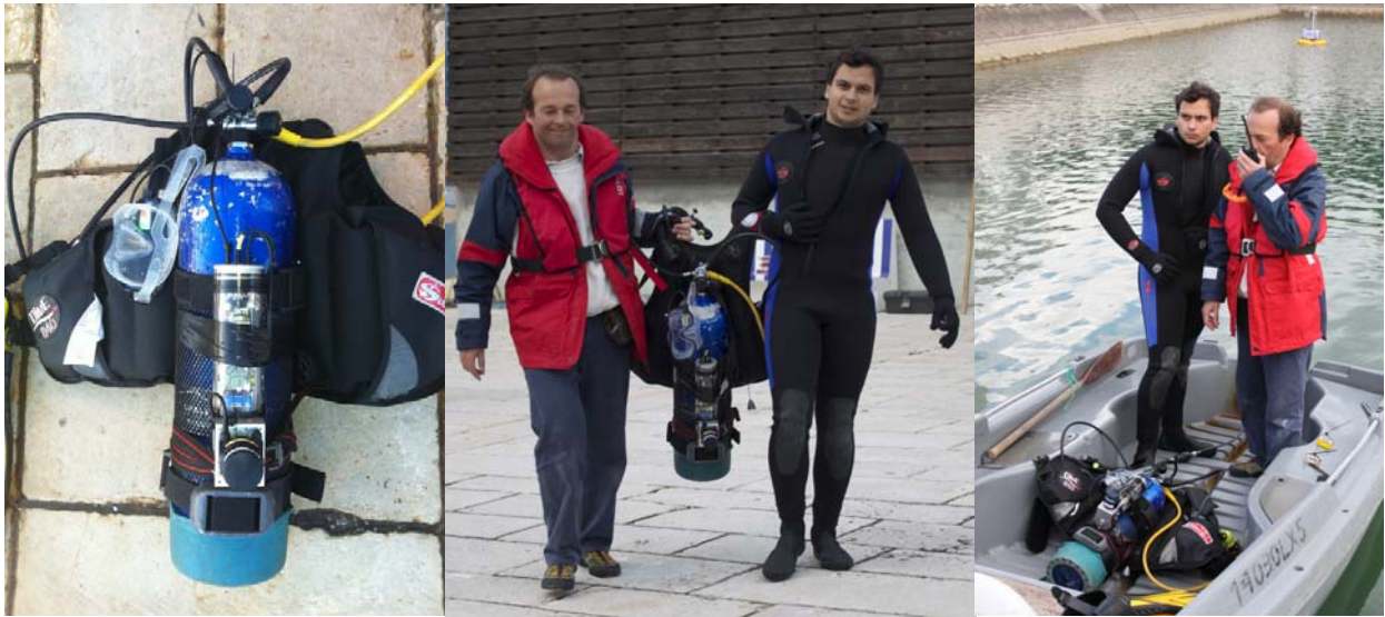
Figure 7. a. Diver unit mounted on the air supply cylinder, b. Diver taking the unit to dive, c. Preparation for the final test
