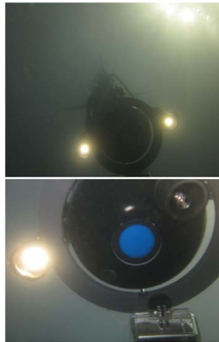
(b) AVP equipped with camera and strobe lights
