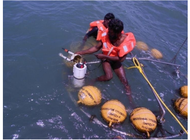
Figure 4. Servicing of mooring assembly and sensor
