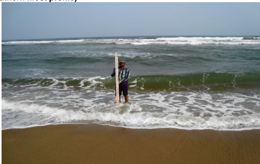
Fig:14. Beach profiling observations under progress near low water line at station:5. ( Southern most profile)
