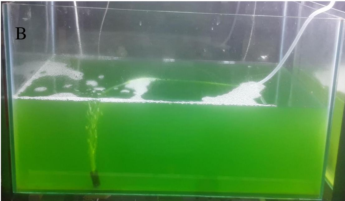
Supplementary Figure 1: Scale up heterotrophic cultivation of Chlorella vulgaris in wastewater enriched medium (A) 0 day and (B) after 4 days of culture duration.
