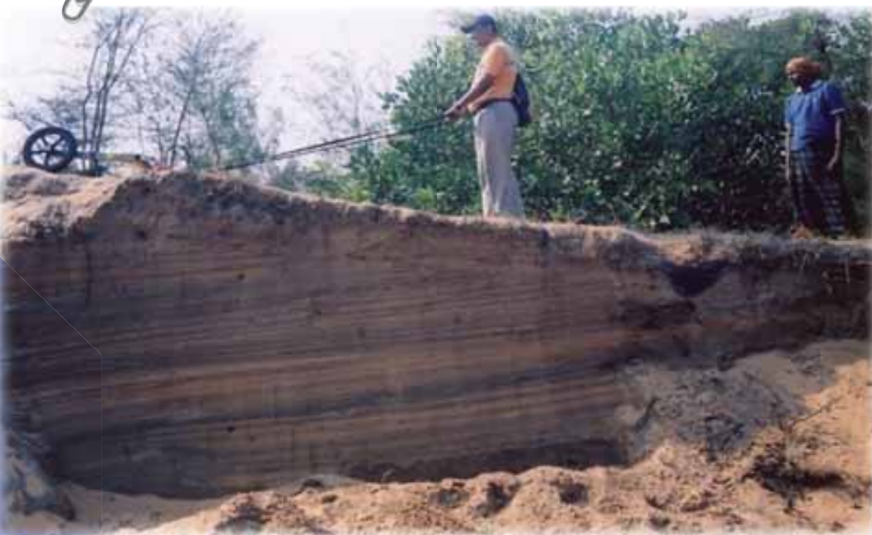
A GPR survey being conducted over a dune cut. Note the garnet-rich sand (brown) alternating with Ilmenite-rich sand (black).
