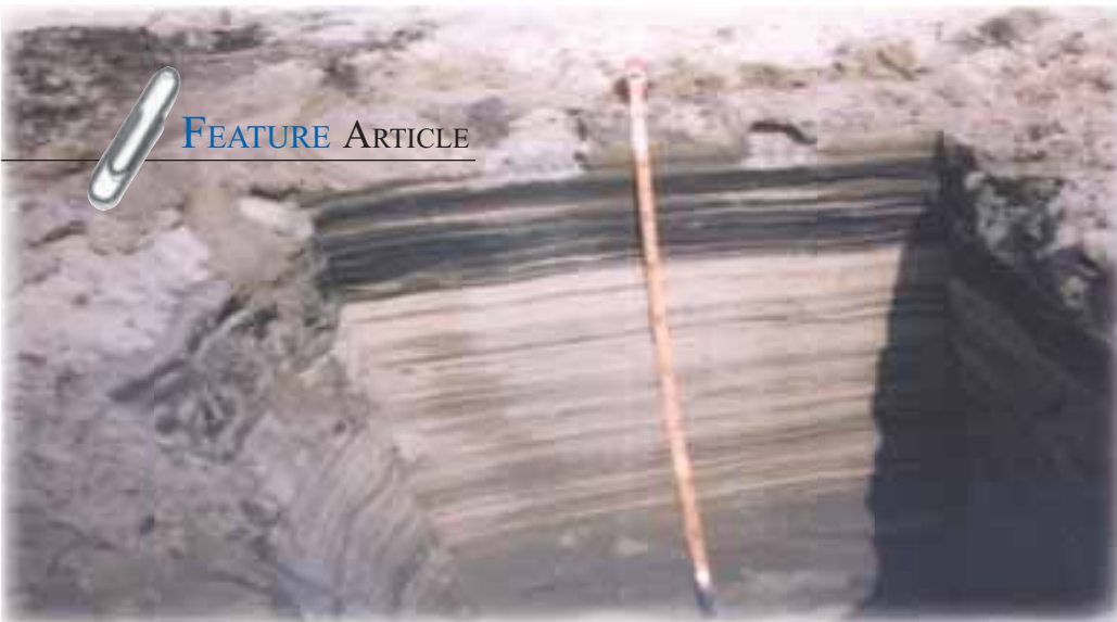
Typical layering of light (quartz) and heavy (ilmenite/magnetite) minerals as noticed in a 1 m depth pit.
